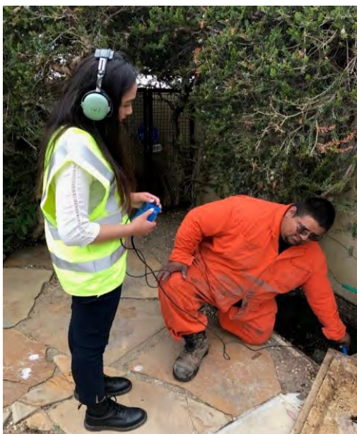
Pinpointing Leaks Using Acoustic Leak Detection Equipment
